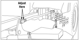
Figure 42. Adjust Lift Rod Timing
